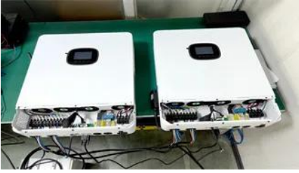
50kW hybrid solar inverter & high-voltage LFP battery
